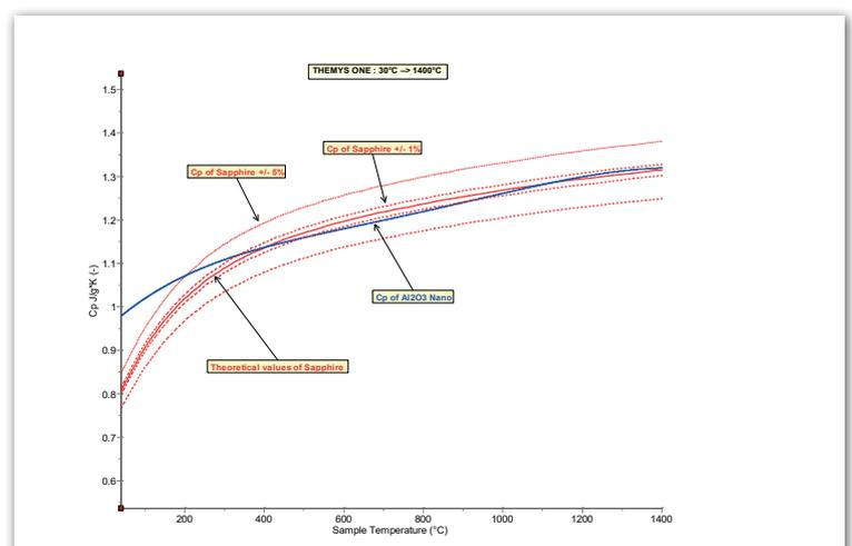
**Figure 4: Cp determination of alumina nanopowder using the continuous heating mode**
