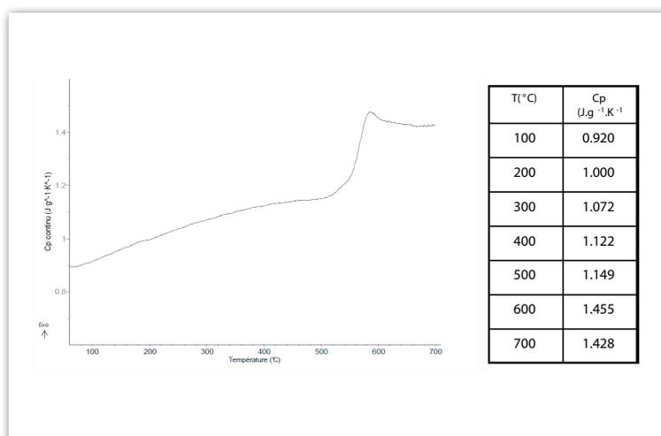
Figure 6:  $C_p$  determination of a glass in the continuous mode
