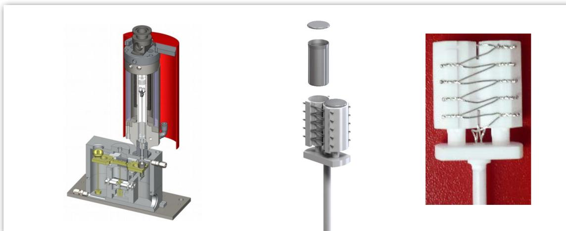
**Figure 1: Cross section of the THEMYS ONE thermoanalyzer and the C<sub>p</sub> 3D DSC detector**
