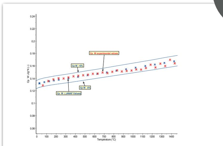
Figure 5:  $C_p$  determination of tungsten in the step heating mode
