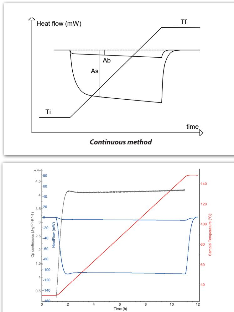
Figure 2:  $C_p$  determination using the continuous heating mode
