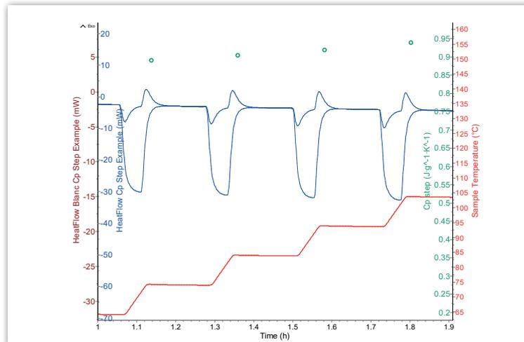
**Figure 3: Cp determination in the step heating mode**
