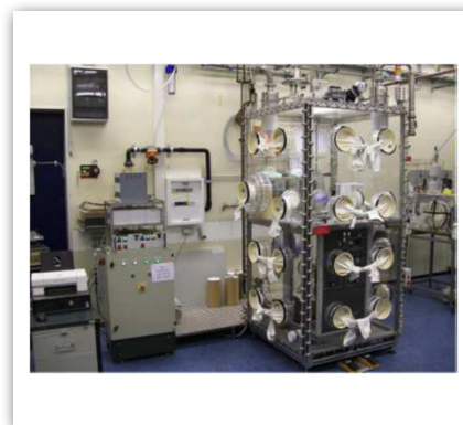
High temperature calorimeter placed in a glovebox (reproduced from [1])
