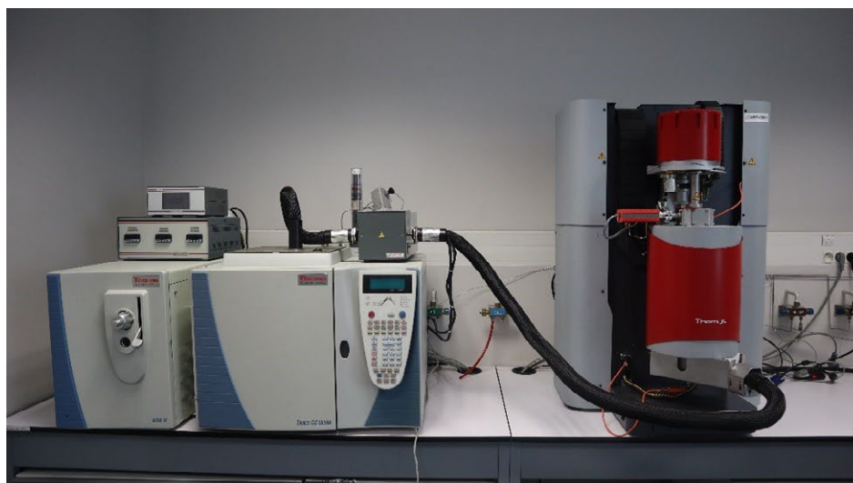
Figure 7: THEMYS thermal analyzer (on the right) coupled with a GCMS (on the left) from ThermoFisher.
