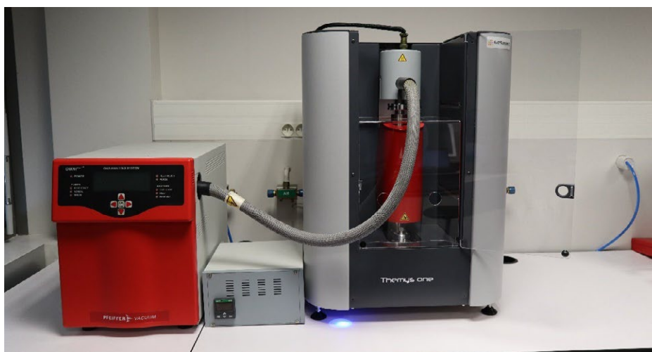
Figure 1: THEMYS ONE thermal analyzer (on the right) coupled with a mass spectrometer (on the left) from Pfeiffer Vacuum.
