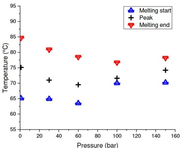
Upon heating, a melting endotherm is measured above 65°C. The onset temperature and the width of the melting peak are modified by the CO<sub>2</sub> pressure.
